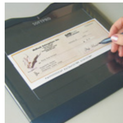
Signing of a transaction form with online capturing of static and dynamic (biometric) characteristics of a signature
