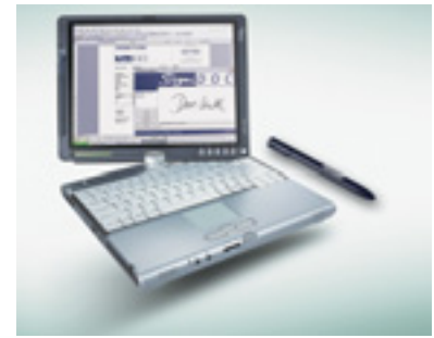
Online capturing of static and dynamic (biometric) characteristics of a signature with a Tablet PC using SignDoc to secure authenticity and integrity of electronic documents
